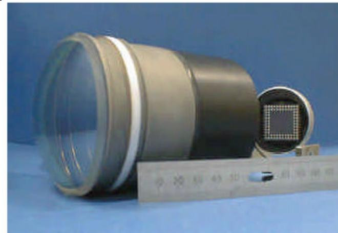
Backup solution using commercial MAPMT, read out by analog pipeline chip (Beetle or SCTA-VELO)
