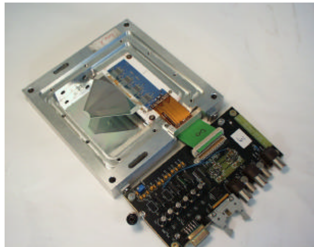
Figure 15: Vertex detector hybrid prototype
