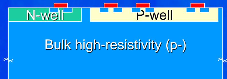
Bulk: all the wafer has rather high resistivity, and twin wells are implanted (n and p wells) on the surface with appropriate dopings for FETs. From about the 130nm node, this type of substrate is used (it is cheaper)
