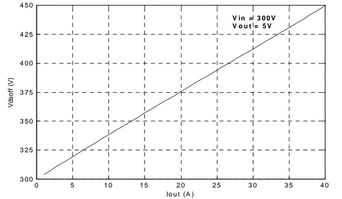
Fig. A1.  $V_{ds_{off}}$  as function of  $I_{out}$  for  $V_{out} = 5V$ , calculated from eqs (2), (a-8) and (a-9).
