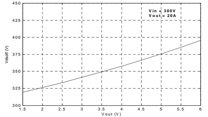
Fig. A2.  $V_{ds_{off}}$  as function of  $V_{out}$  for  $I_{out} = 20A$ , calculated from eqs (2), (a-8) and (a-9).
