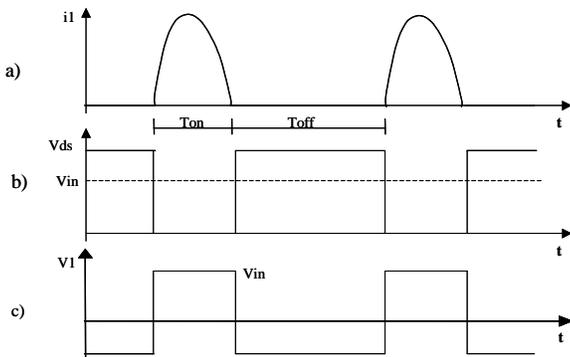
Fig. 2. Switch current  $i_l$  (a) and drain-source  $V_{ds}$  (b) as function of time for the power transistor  $Q$ . Voltage waveform of the transformer primary winding (c).
