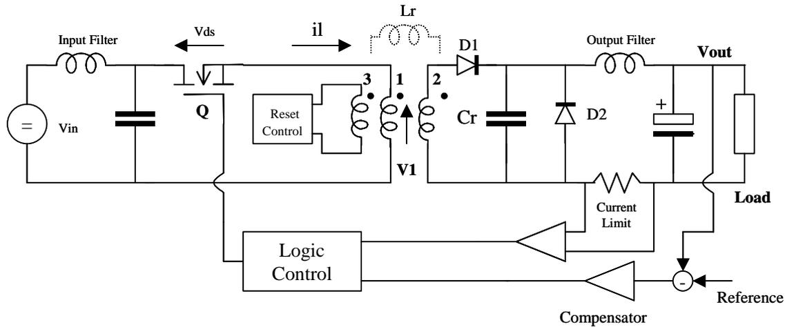
Fig.1. Schematic diagram of the VICOR DC-DC converter. The inductor  $L_r$  represents the series parasitic inductance of the transformer; Dots ( $\bullet$ ) are used to indicate points on the transformer schematic symbol that have the same instantaneous polarity.
