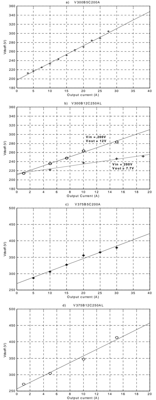
Fig. 3.  $V_{ds_{off}}$  of the power transistor Q as function of the output current with the converter operating at reduced input voltage. a) Converter V300B5C200A,  $V_{in} = 200V$ ; b) Converter V300B12C250AL,  $V_{in} = 200V$ ; c) Converter V375B5C200A,  $V_{in} = 260V$ ; d) Converter V375B12C250AL  $V_{in} = 260V$ .
