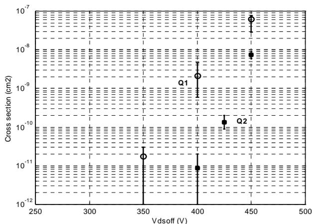
Fig. 4. 60MeV protons cross section for Q1 (open symbols) and Q2 (closed symbols) power MOSFETs, both rated 600V/6A. Error-bars depict the minimum and maximum cross sections
