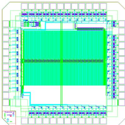
Figure 2: Layout view of the memory chip.
